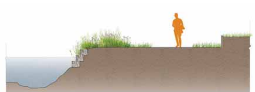
Edge treatment - Gabion Box
