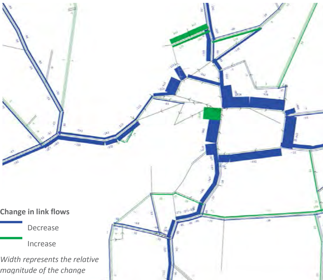
Figure 3.17 Changes in link flows between the 2031 future baseline model and 2031 Scenario 8 model, AM peak hour
