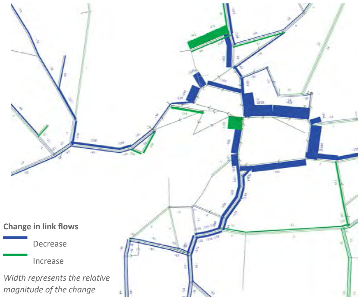
Figure 3.21 Changes in link flows between the 2031 future baseline model and 2031 Scenario 8 model, PM peak hour
