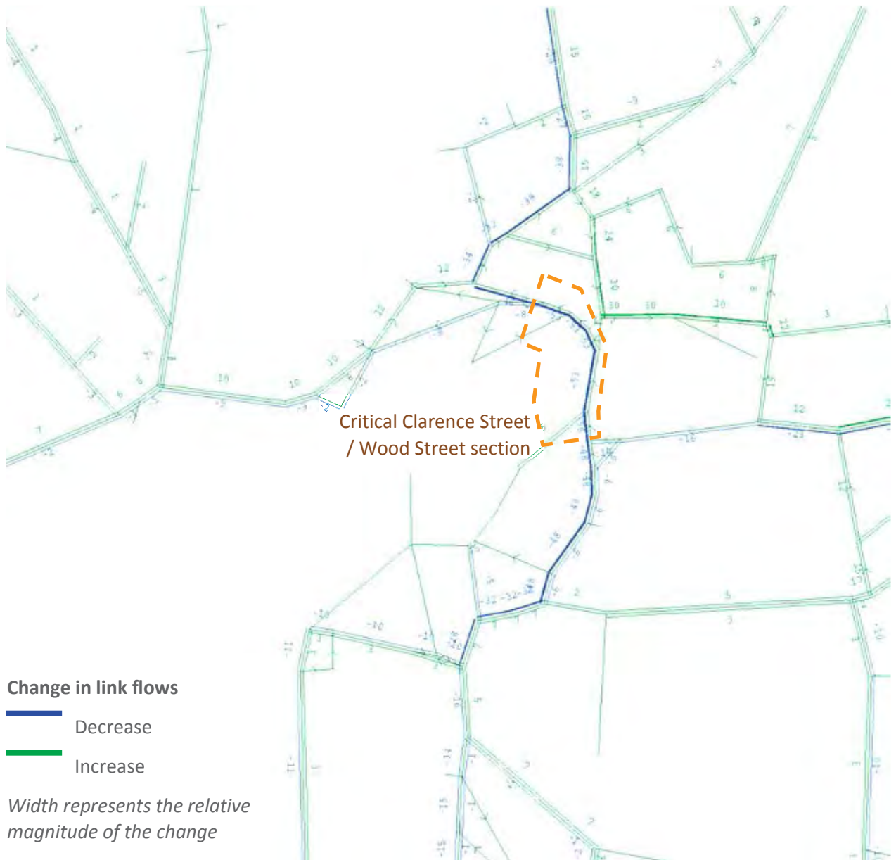
Figure 3.7 Changes in link flows between the 2031 future baseline model and 2031 Scenario 1 model, PM peak hour
