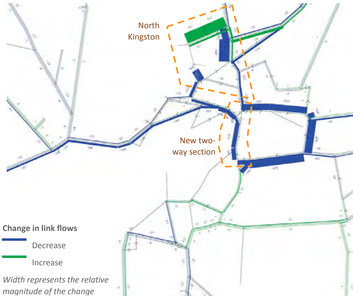
Figure 3.9 Changes in link flows between the 2031 future baseline model and 2031 Scenario 3 model, AM peak hour
