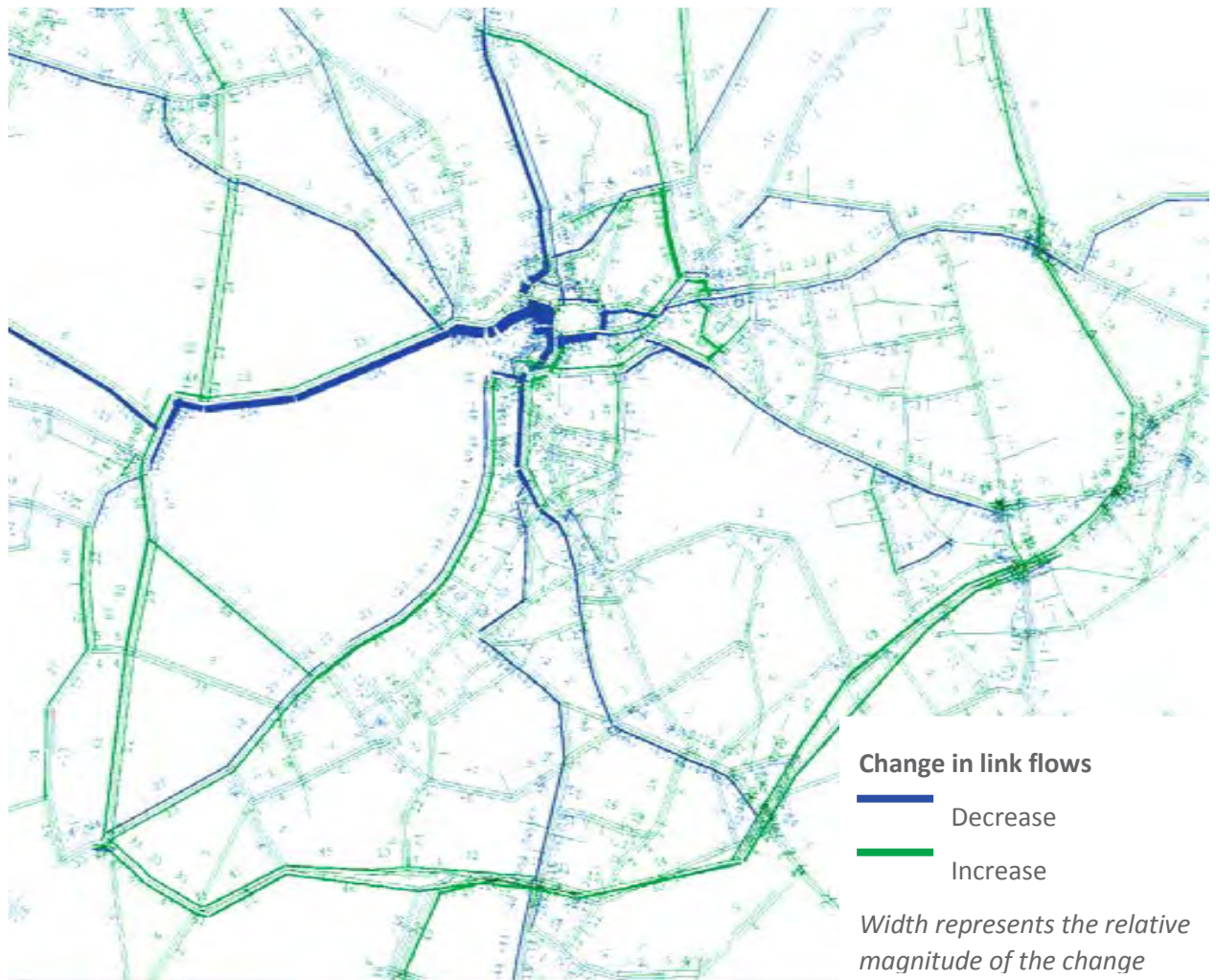
Figure 3.5 Changes in link flows between the 2031 future baseline model and 2031 Scenario 1 model, AM peak hour, wider area
