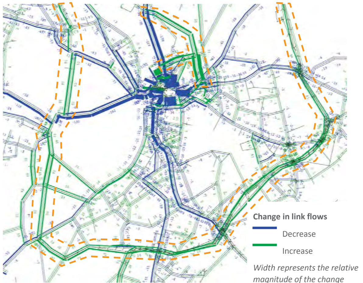
Figure 3.20 Changes in link flows between the 2031 future baseline model and 2031 Scenario 8 model, AM peak hour, wider area
