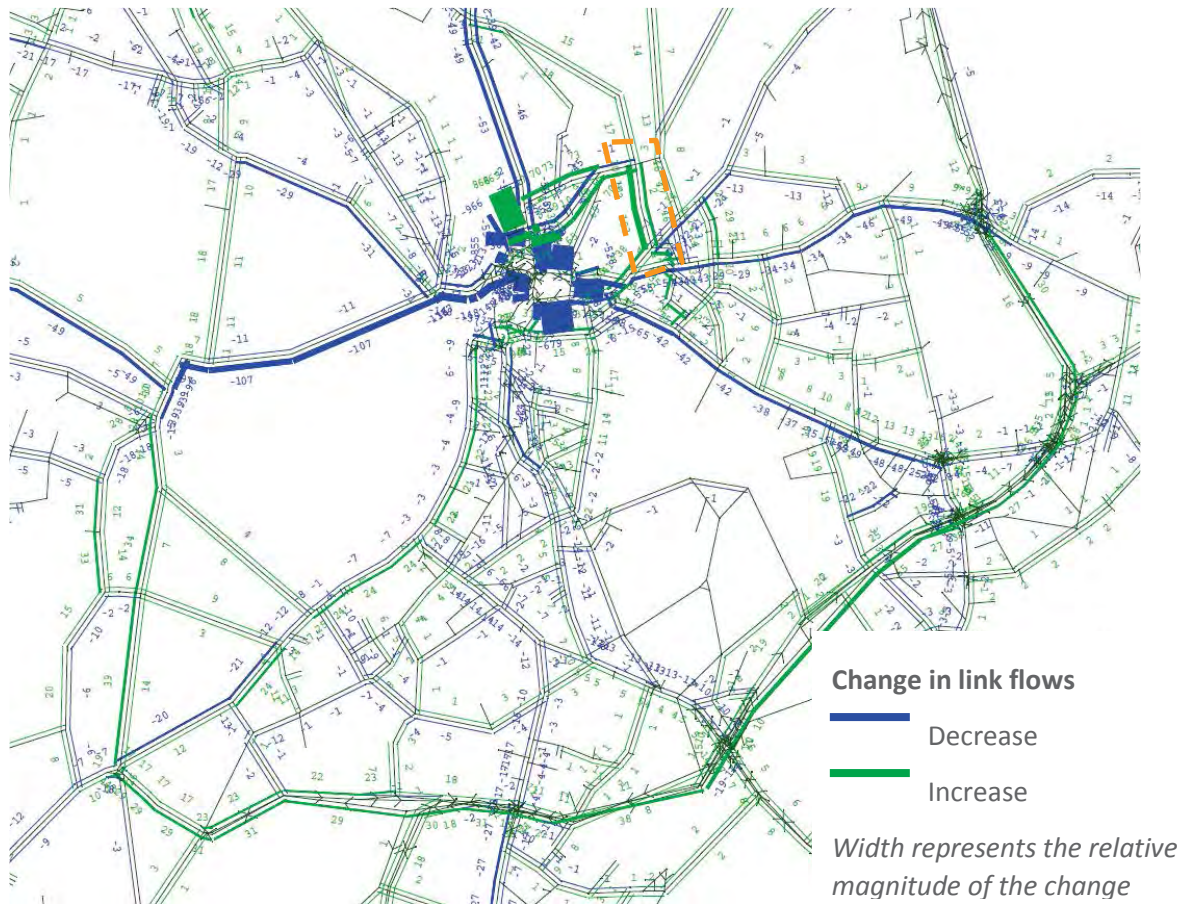
Figure 3.12 Changes in link flows between the 2031 future baseline model and 2031 Scenario 3 model, AM peak hour, wider area
