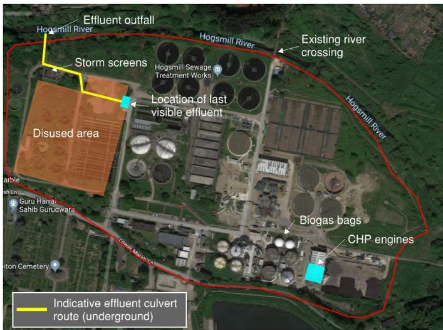
Figure 9-1 Annotated Hogsmill WWTP site map
