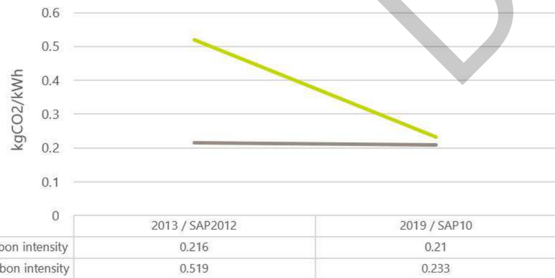
Figure 3.4: Fuel carbon intensities as per SAP 2012 and SAP 10
