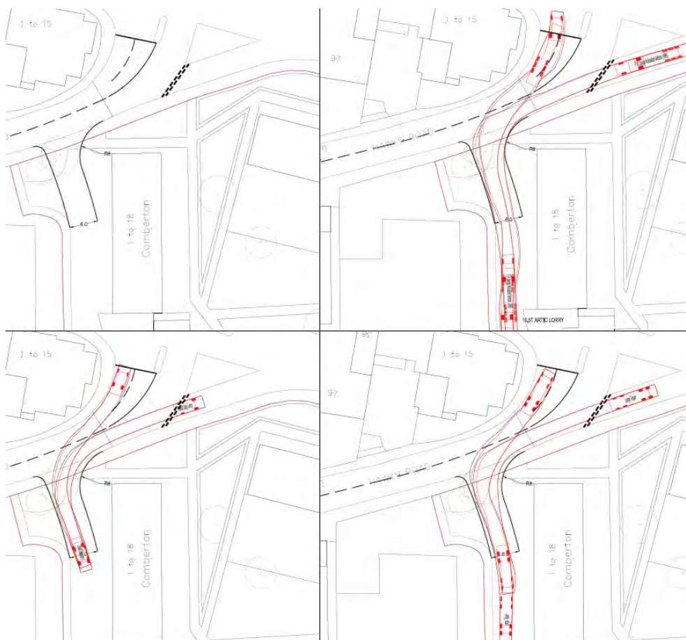
Image 7.1 Phase 1 Hawks Rd Access – Swept Path Analysis
