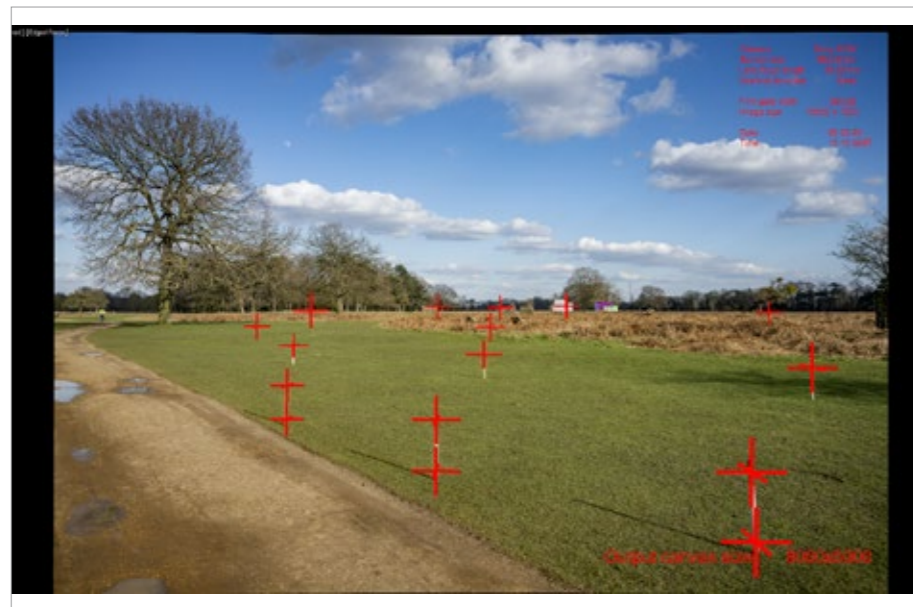
3.7 Screen grab of model matched to photograph
