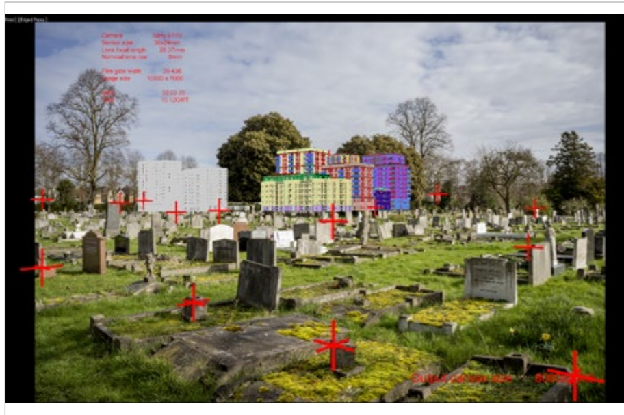
3.7 Screen grab of model matched to photograph
