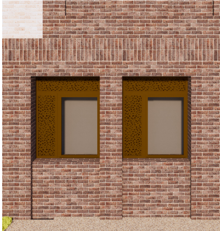
Figure 4.36: Ventilation panels incorporated into window assembly - Fixed perforated panels with internal opening casement.
