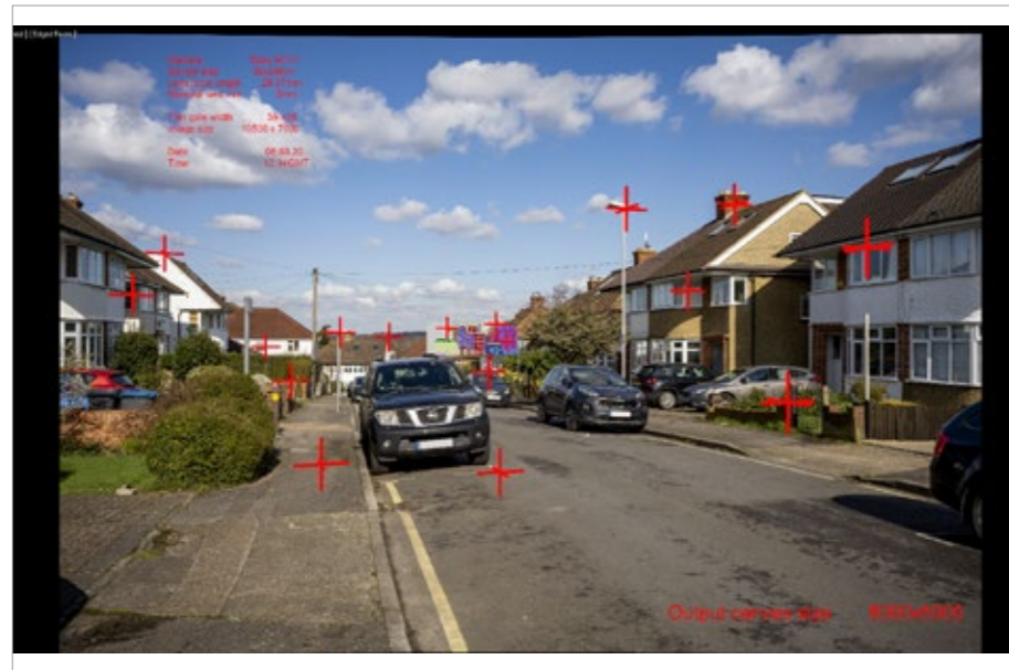
3.7 Screen grab of model matched to photograph
