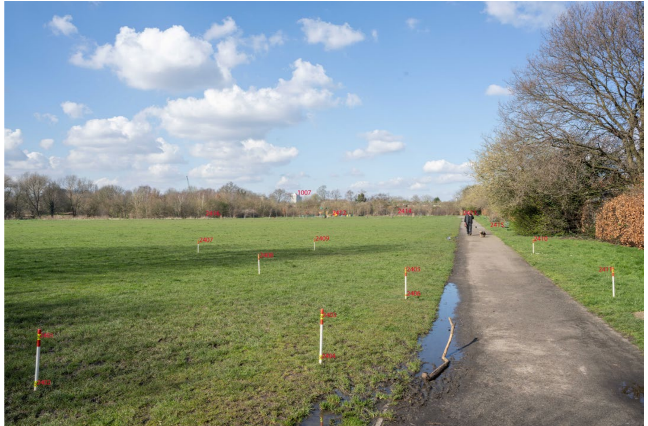
3.2 OS survey points marked on base photograph
