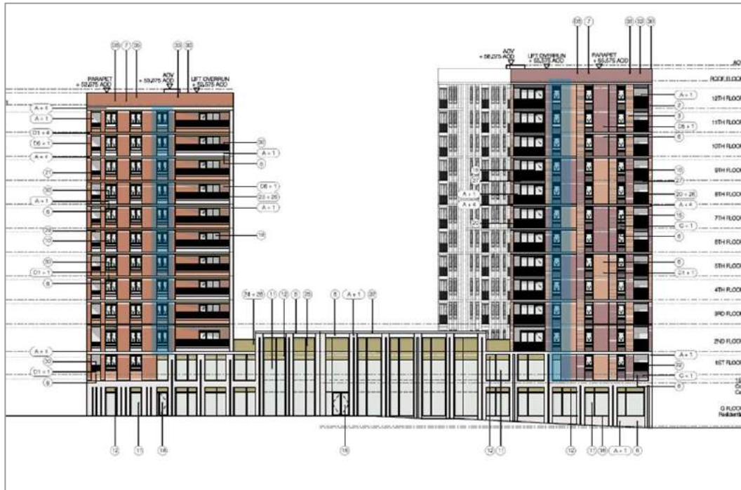
Figure T5.5. Blocks C1 & C2, west elevation. Windows that require blinds are marked up in blue (Patel Taylor drawings 23.10.2020).
