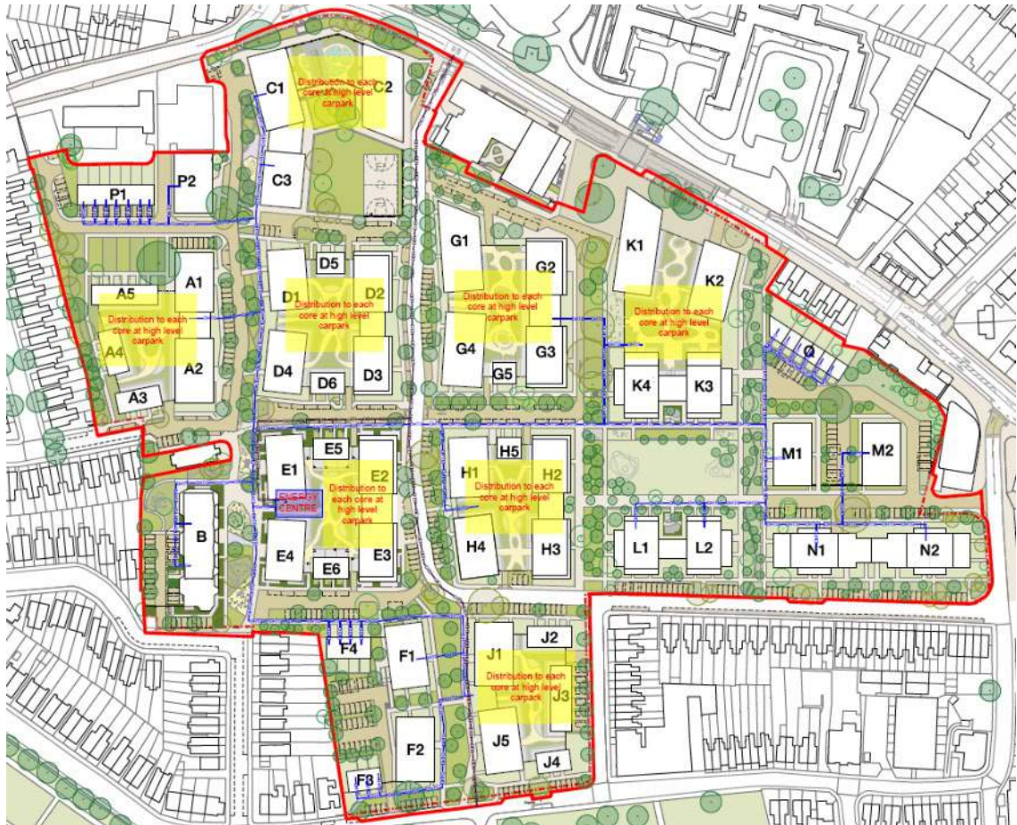
Figure 7: Cambridge Road Estate Heat Network with DEN connection courtesy of AWA Building Services Consultants
