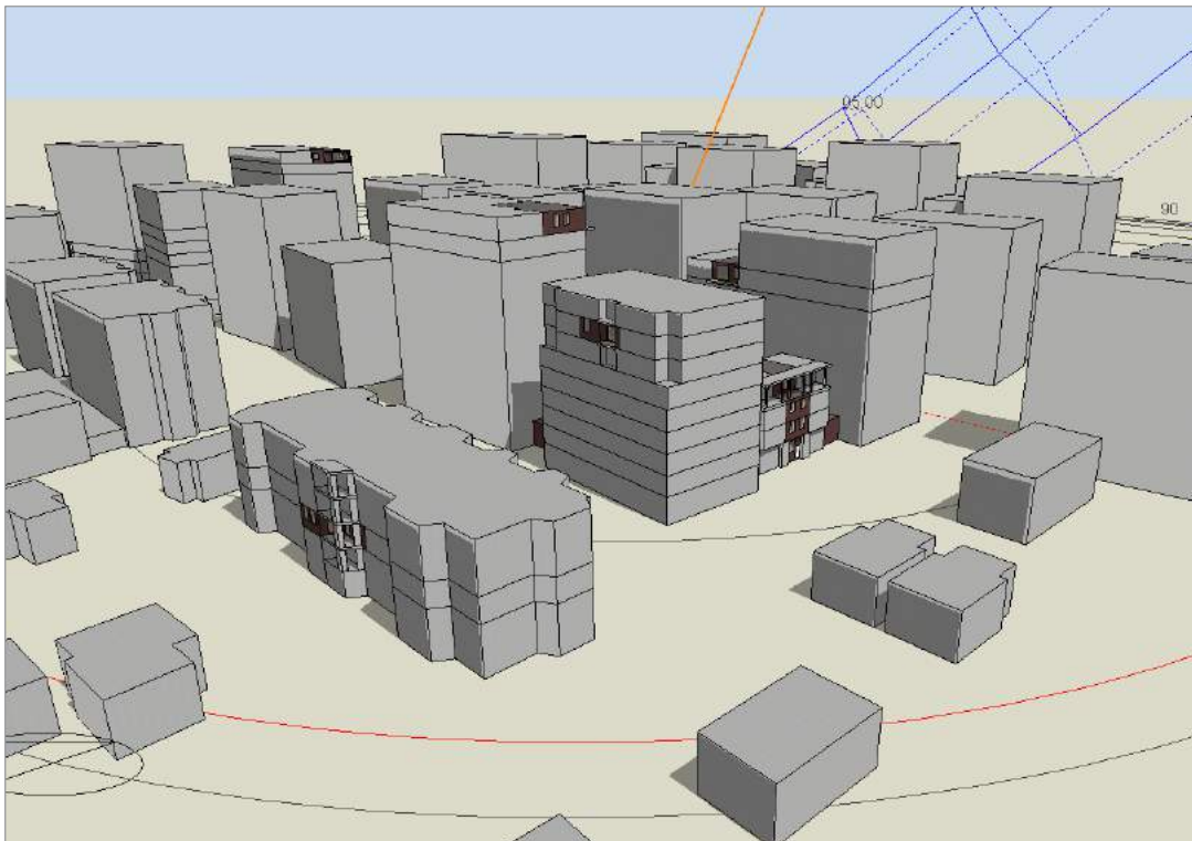
Figure 4: Design builder simulation model for Blocks B and E, sun path shown for 21 st June 12:00 noon BST.
