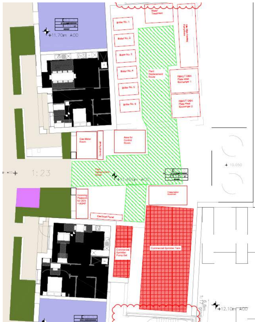
Figure 8: Indicative Block E energy centre layout courtesy of AWA Building Services Consultants
