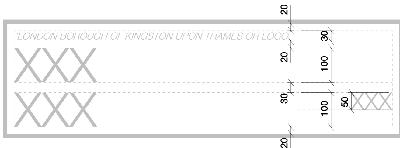
Figure 4.108: Example of street naming signage setting out.
