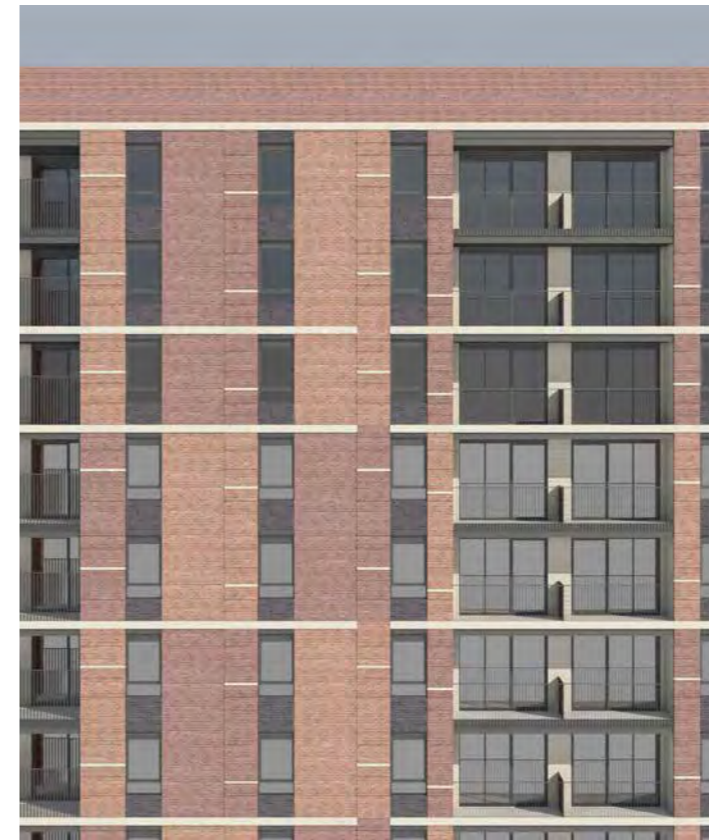
Figure 97: Proposed brickwork of C1
