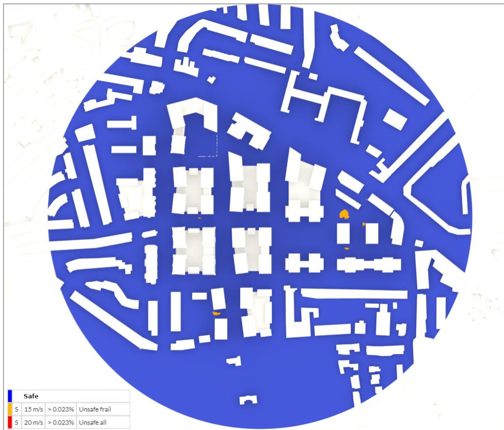
Figure 2 - Lawson Safety Conditions. Result for the whole year, scenario 2. 1.50m above the ground
