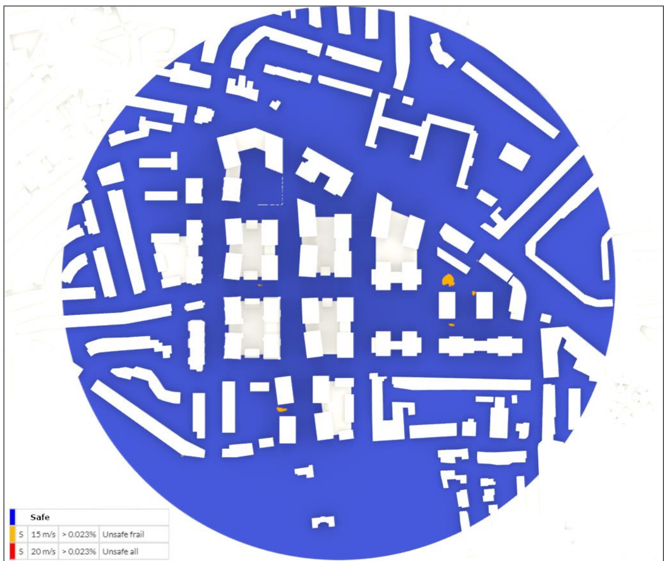
Figure 19 - Lawson Safe Conditions. Proposed Development, scenario 2, result for the whole year. 1.50m above the ground
