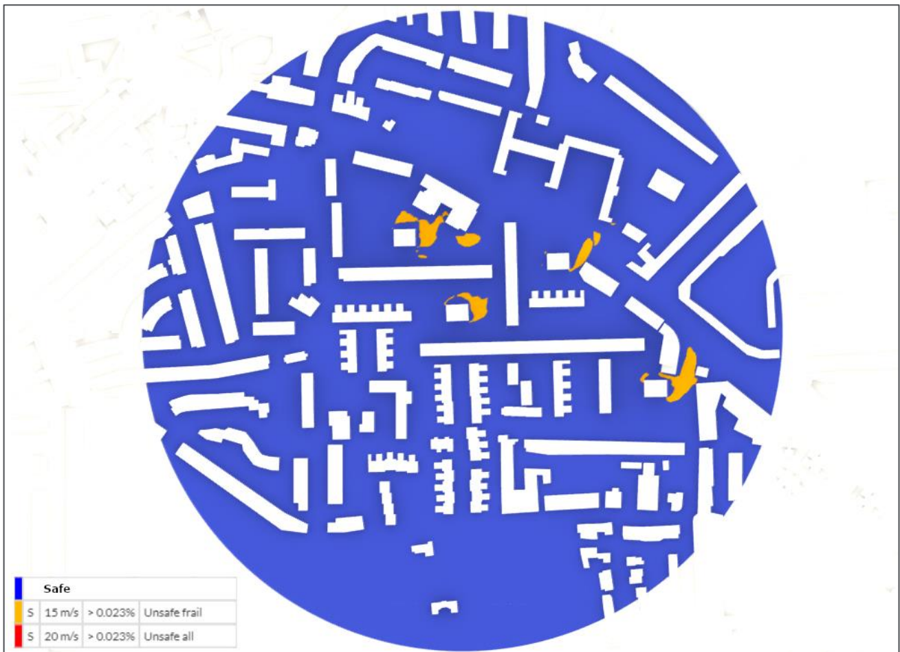
Figure 13 - Lawson Safe Conditions. Existing conditions, scenario 1, result for the whole year. 1.50m above the ground
