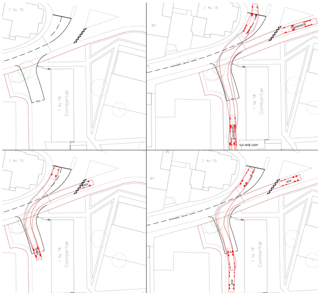
Image 0.1 Phase 1 Hawks Rd Access – Swept Path Analysis
