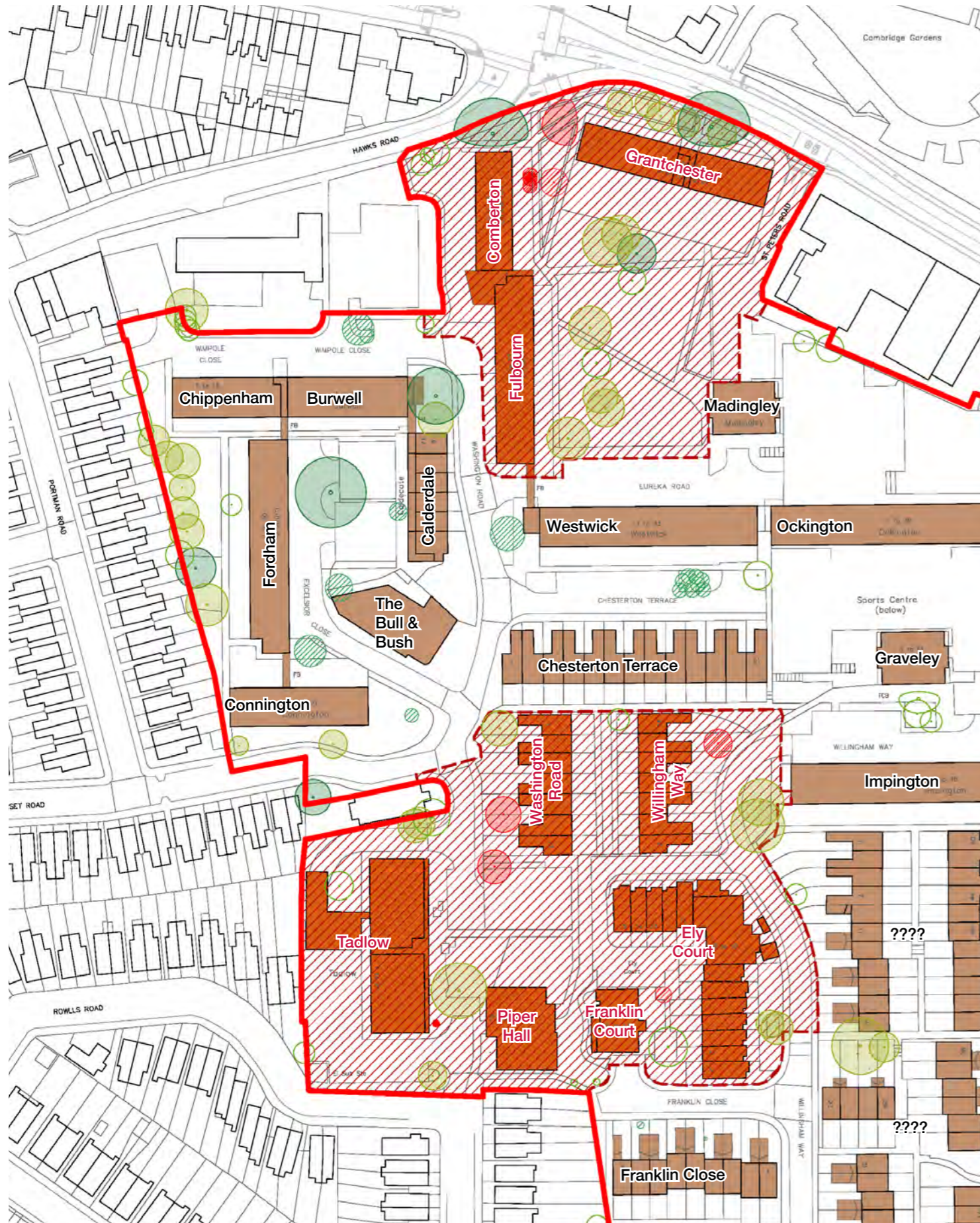
Figure 10: Scope of Initial site clearance and demolition.
