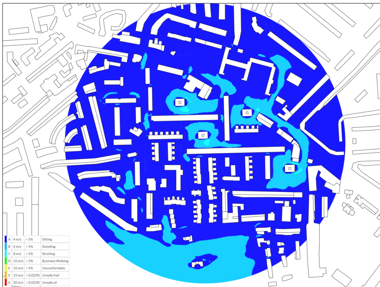
Figure 13 - Lawson Safe Conditions. Existing conditions, scenario 1, result for the summer season. 1.50m above the ground
