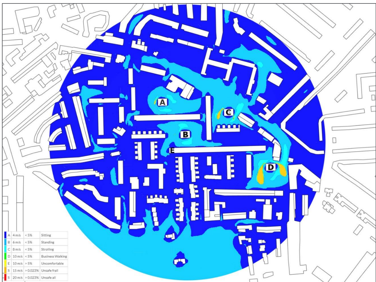
Figure 12 - Lawson Safe Conditions. Existing conditions, scenario 1, result for the windiest, winter season. 1.50m above the ground
