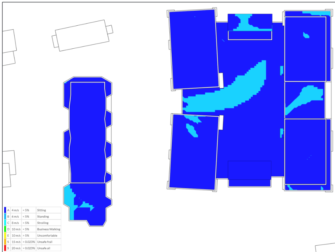
Figure 20 - Lawson Safe Conditions. Proposed Development, scenario 2, result for the podium level and roof terraces at block B and E, summer season. 1.50m above floor level
