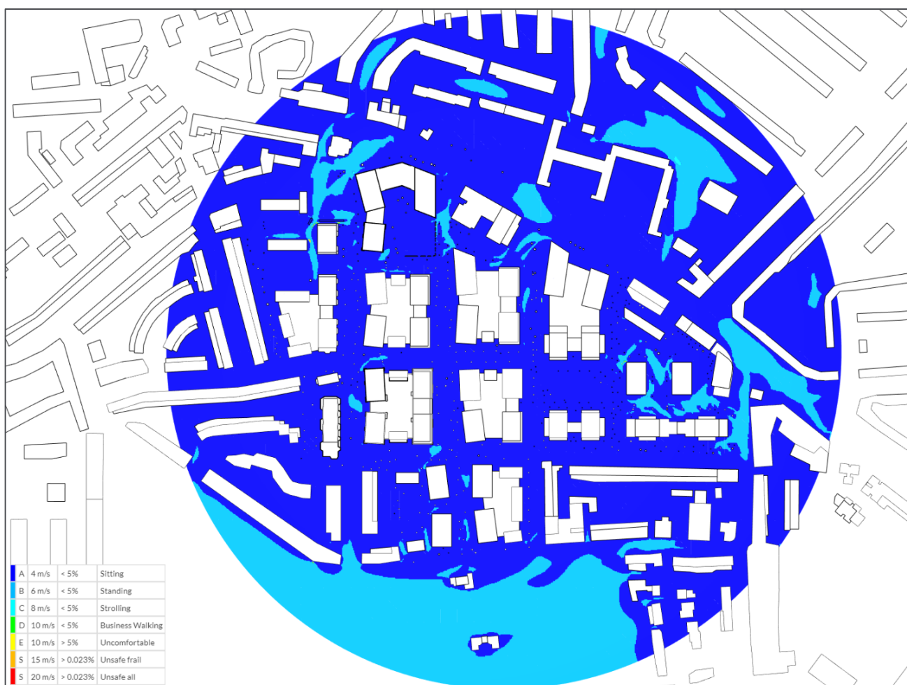
Figure 23 - Lawson Safe Conditions. Proposed Development, scenario 2, result for the winter season. 1.50m above the ground
