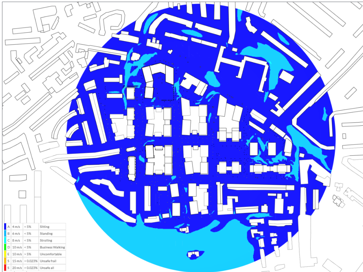
Figure 2 - Lawson Safety Conditions. Result for the windiest, winter season, scenario 3. 1.50m above the ground
