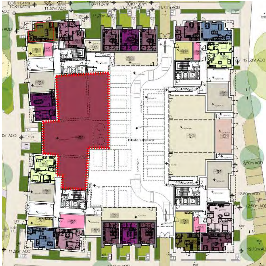
Figure 10: Energy Centre Below Podium in Block E
